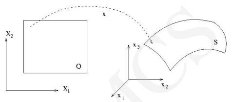
Fig. 1. Parametric representation of a surface
