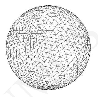
Fig. 8. Unstructured mesh on a sphere
