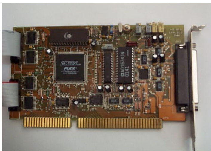
Fig. 3. The analog-digital card ADC615
