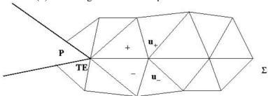
Fig. 2. The Kutta-Zhukovsky condition on slit  $\Sigma$
