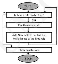
Fig. 1. The scheme of forward chaining
