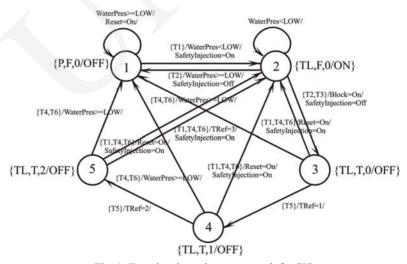
Fig. 1. Functional requirements graph for SIS
