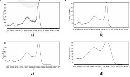
Fig. 5. The fuzzy entropy histogram of one of MR slices for various bandwidths: the original histogram (a), the fuzzy histogram with the bandwidth  $\Delta b$ =5 (b),  $\Delta b$ =15 (c),  $\Delta b$ =40 (d)
