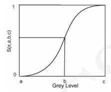
Fig. 1. Graph of the standard S-function, b=(a+c)/2, bandwidth  $\Delta b=b-a=c-b$  and k=2
