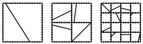
Fig. 1. Dyadic partitions on different levels of decomposition with arbitrary beamlets
