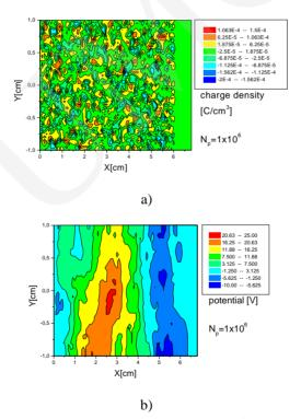
Fig. 4. Charge density and potential distribution obtained for 10<sup>6</sup> macro-particles distributed homogeneously in a rectangular box
