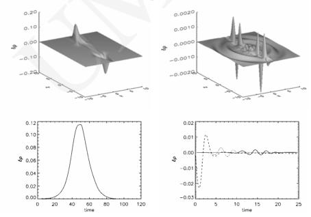
Fig. 2. The spatial profile of the perturbed mass density  $\delta\rho(x, y = 0, z, t)$  (top panels) and the time-signetures (bottom panels) which is obtained by measuring the wave signal in  $\delta\rho$  at a fixed spatial location
