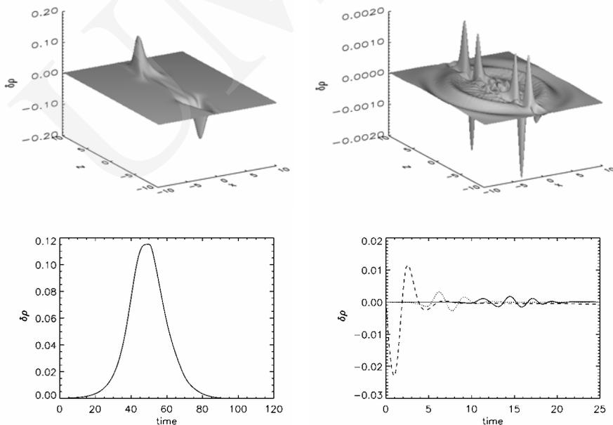
Fig. 2. The spatial profile of the perturbed mass density  $\delta\rho(x, y = 0, z, t)$  (top panels) and the time-signatures (bottom panels) which is obtained by measuring the wave signal in  $\delta\rho$  at a fixed spatial location
