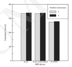
Fig. 2. The execution time as a function of different compilation options for MPI in the case of 2 or 4 running processes
