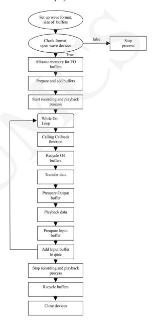
Fig. 3. The flow chart of the delaying algorithm of the speech echo-corrector
