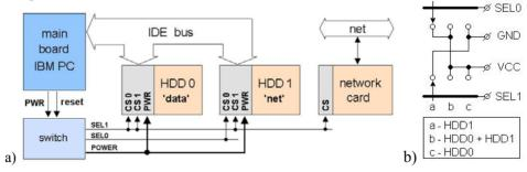
Fig. 5. Scheme of control connection of the HDD disk and network card switches (a) and scheme of mechanical switch (b)
