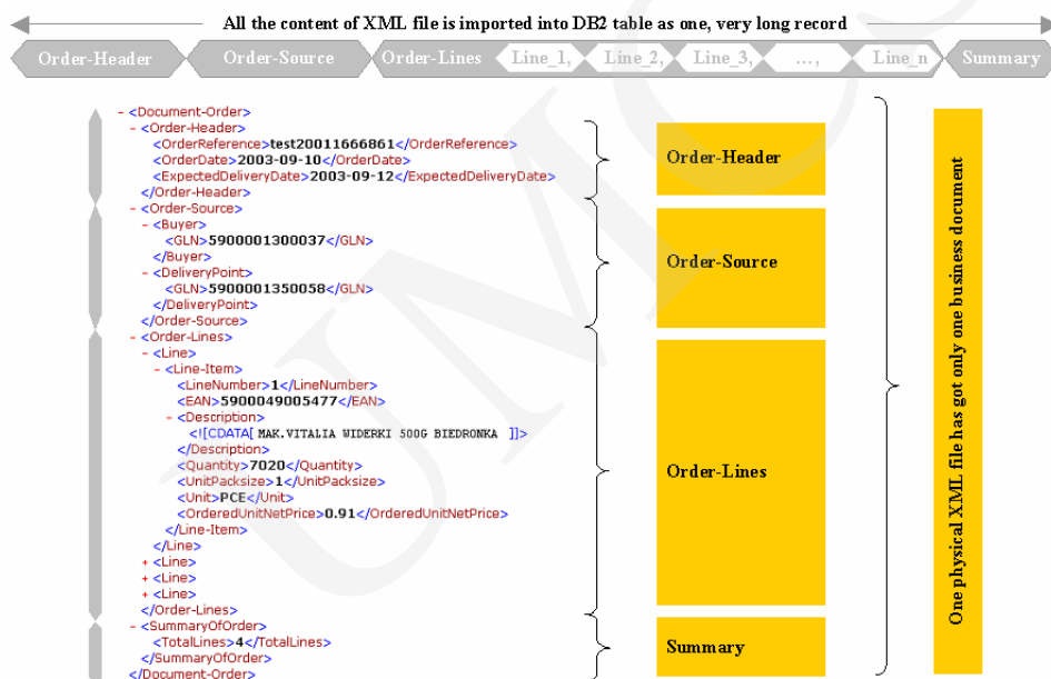
Fig. 3. The logical structure of the XML file example - provided by firm B
