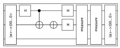
Fig. 2. Deutsch's algorithm drawn by the QCL2eps program
