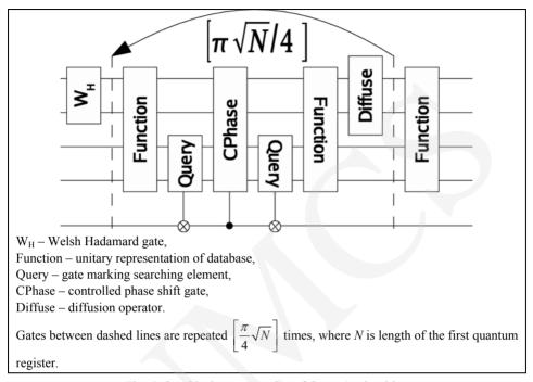
Fig. 6. Graphical representation of Grover's algorithm
