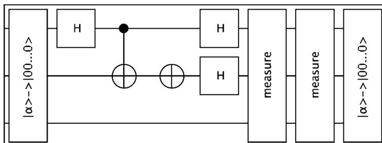
Fig. 2. Deutsch's algorithm drawn by the QCL2eps program
