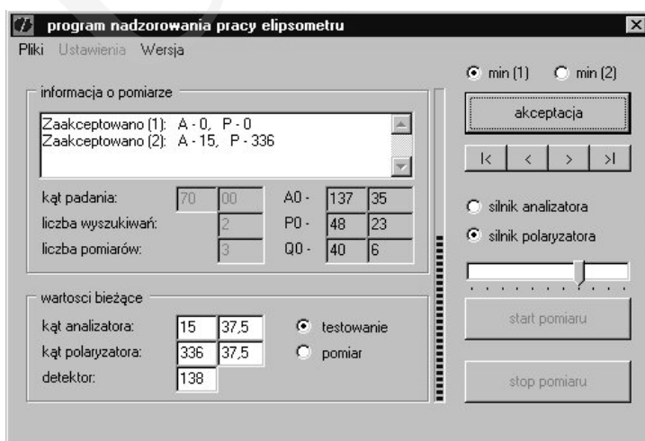
Fig. 4. Ellipsometer operation management program – graphical interface
