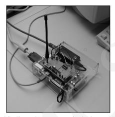
Fig. 9. Testbed for direct wireless communication between FPGA devices
