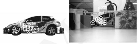
Fig. 8. Interest points automatically matched in a model image and a camera-captured view
