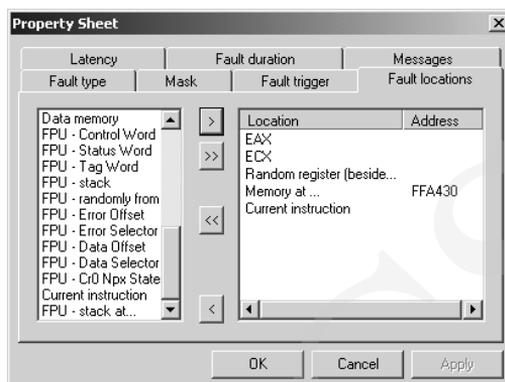
Fig. 1. FITS window for defining fault injections
