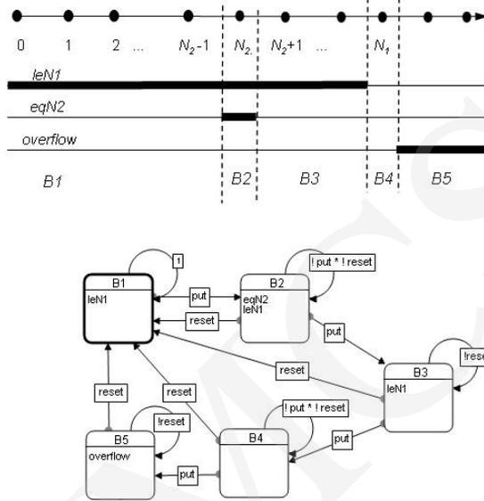
Fig. 2. CSM model of Buffer for  $N_1 > N_2$
