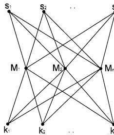
The degree of cohesion of the graph equals  $d = |E| - |V| + 1 = rm + nm - r - n - m + 1 = (r + n - 1)(m - 1)$ . If we compare this topology with the previous one (in the previous topology  $m = 1$  and  $d = 0$ ), the degree of reliability increases  $m - 1$  times for this SK. The algebraical notation for this topology:
