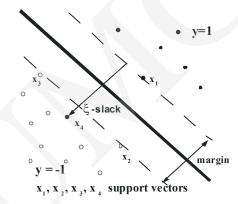
Fig. 1. Hyperplane classifier in two dimensions. Points  $x_1$ ,  $x_2$  and  $x_3$  define the margin, i.e. they are the support vectors
