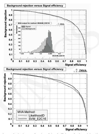
Fig. 5. The background rejection as a function of signal efficiency for the training (dashed line) and test (solid line) for the simulated ATLAS  $\tau$  data while using SVM (left plot). Also the distributions of the discriminants for signal and background are shown. The SVM method (solid line) is compared with the likelihood estimator (dotted line) (right plot)
