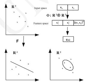
Fig. 2. Example of data separable by an elliptic curve in  $\Re^2$ , but linearly separable in the feature space  $\Re^3$ . The mapping to transforms  $(x_1, x_2) \to (x_1^2, x_2^2, \sqrt{2}x_1x_2)$ .
