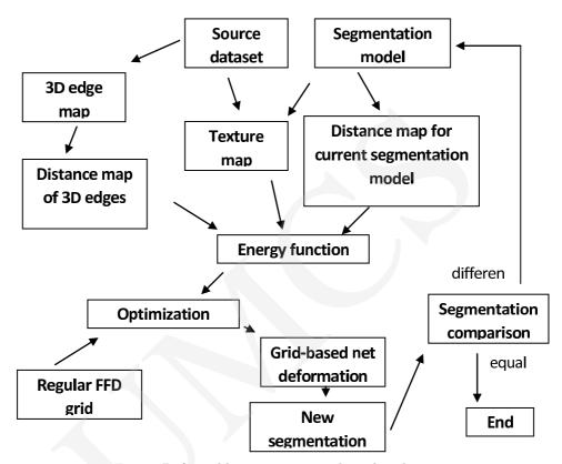
Fig. 2. Deformable segmentation algorithm diagram
