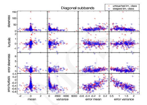
Fig. 5. Scatter plots of tested images from two classes: untouched image class and stegoed image class
