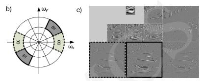
Fig. 1. Steerable pyramid transform: a) – the transformation filter structure, b) – the Fourier magnitude spectrum with marked frequencies passed by the filters  $B_0$  and  $B_1$ , c) – two levels of a sample image decomposition with four filtering directions
