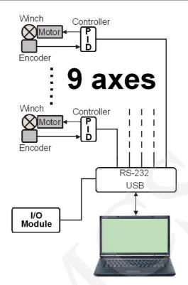
Fig. 5. The architecture of control system
