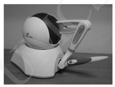
Fig. 7. The PHANTOM Omni haptic device
