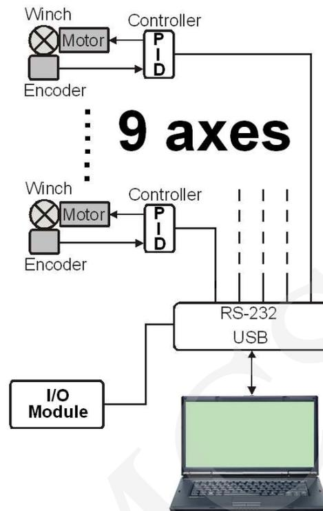
Fig. 5. The architecture of control system
