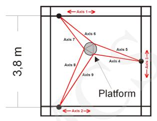
Fig. 3. The top view on the 9-DOF robot
