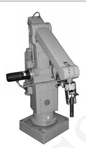
Fig. 1. 5–DOF robotic arm with the gamma radiation detector – the example of the use of the standard manipulator arm for manipulations in radioactive environments
