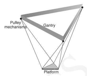
Fig. 2. Simplified scheme of the cable-driven manipulator system
