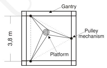
Fig. 3. Axonometric projection of the cable-driven manipulator system
