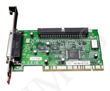
Fig. 2. Adaptec AVA 2906 controller.
