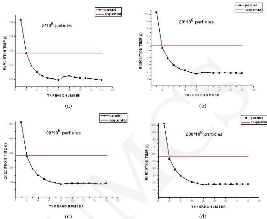
Fig. 3. Time of charge density calculations as a function of the number of threads used for the parallel run, using the NGP method, mesh of size  $100 \times 100 \times 100$  and a different number of macro particles: a) 2mill, b) 20mill, c) 100mill, d) 200mill.
