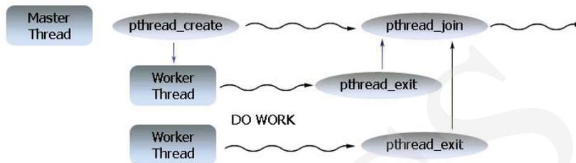
Fig. 2. Threads synchronization.
