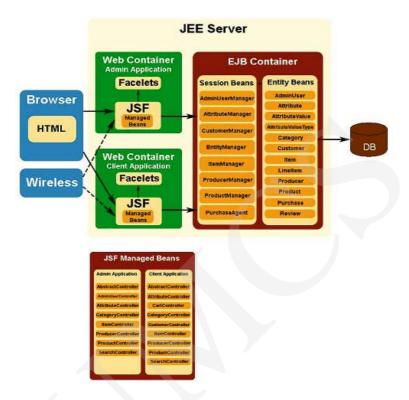
Fig. 1. System architecture.
