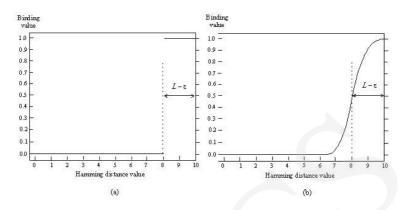
Fig. 5. Relation between the binding value and the match score (in the case of the Hamming distance) for a bit-string of length L=10 and affinity threshold  $\varepsilon=2$ . (a) Threshold binding function. (b) Sigmoid binding function (the picture is based on the information provided in [10]).
