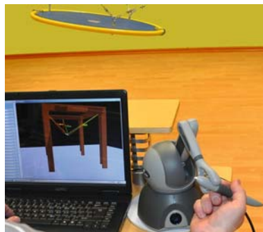
Fig. 9. The control of the cable manipulator system by means of the haptic.
