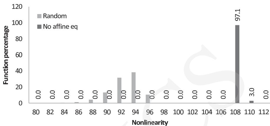
Fig. 7. Nonlinearity of S-boxes with removed affine equivalence.
