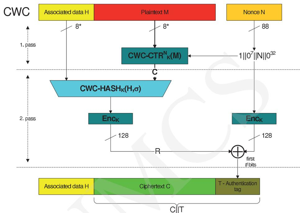
Fig. 5. CWC authenticated encryption scheme.
