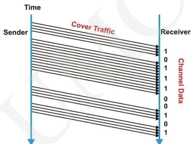
Fig. 4. Idea of timing based covert channels.
