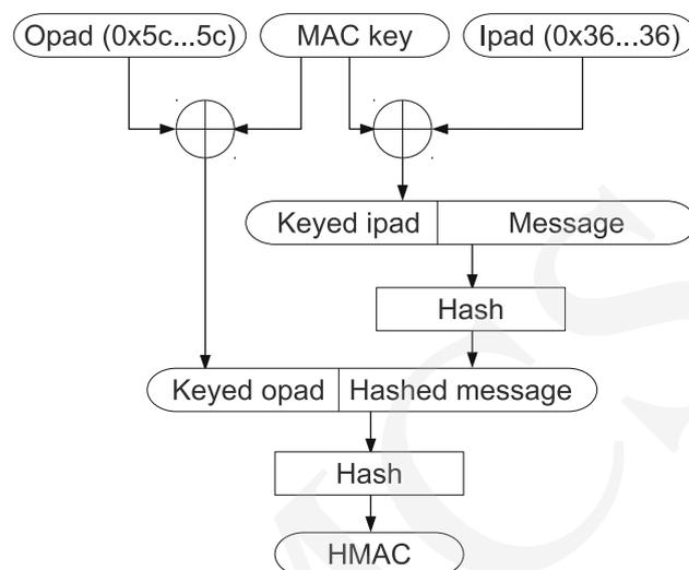
Fig. 11. HMAC calculation.
