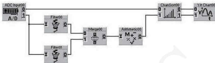
Fig. 2. Filtering, adjusting and amplifying the signal.
