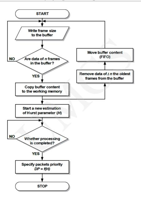
Fig. 6. Priority Management Module algorithm.
