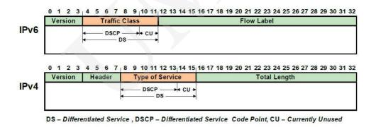
Fig. 1. DSCP field in the header of IPv6, and IPv4 packets.
