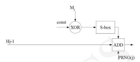
Fig. 6. StreamHash 2 NLF mini-transformation scheme while using a correct internal state for the attack.
