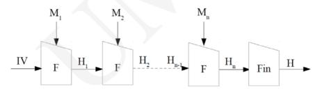
Fig. 1. StreamHash mode of operation.
