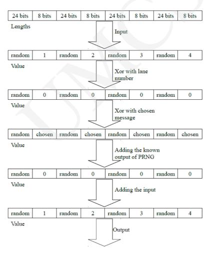
Fig. 5. Data flow in the compression function.
