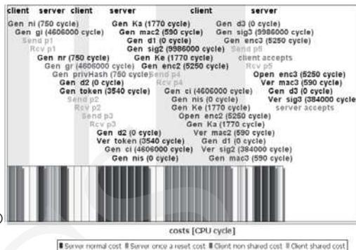
Fig. 7. *SigmaI* protocol specification fragment and protocol run visualization in the *DoS Analyzer* system.
