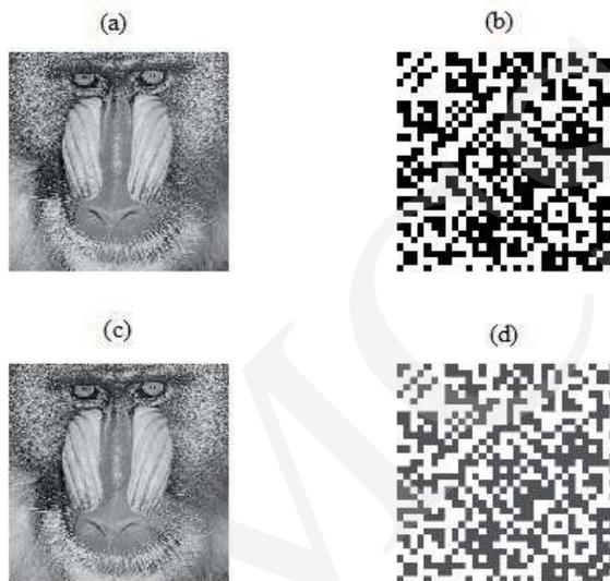
Fig. 2. Simple watermarking scheme in DWT domain, original image (a), watermark (b), watermarked image (c), extracted watermark (d).
