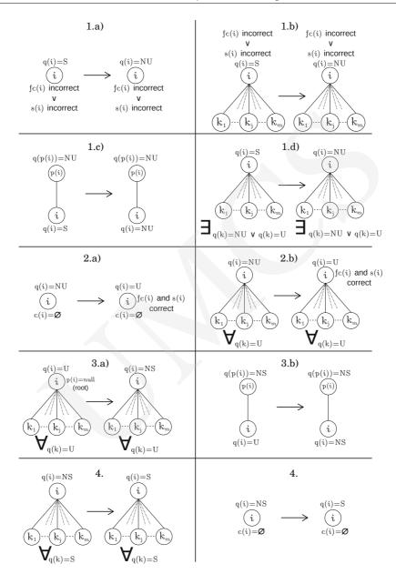
Fig. 2. An illustration of the ASFC II algorithm rules, where  $k \in c(i)$ .
