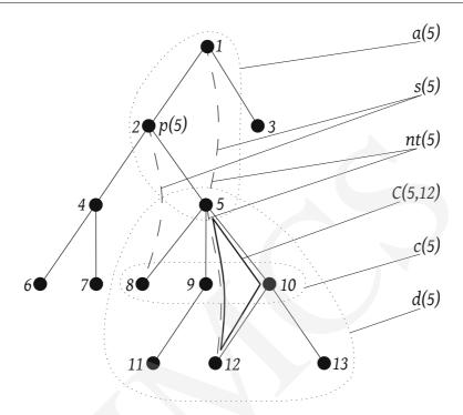
Fig. 1. Illustration of the notation for the node i=5:  $n(5)=\{1,2,8,9,10,12\}$ ,  $su(5)=\{\{2,8\},\{5,12\}\}$ ,  $fc(5)=\{\{1,5\},\{2,8\},\{5,12\}\}$ . Dashed lines indicate the nontree edges. Solid lines indicate the tree edges.
