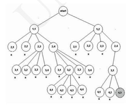
Fig. 1. Description of the return-Tree(backtracking) [3].
