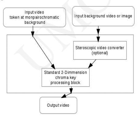
Fig. 1. Stereoscopic video processing block scheme.
