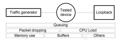
Fig. 1. Stress test – connection diagram.
