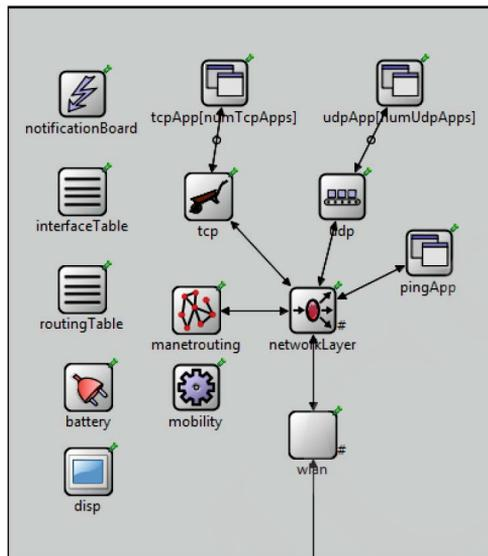
Fig. 11. Wireless sensor network node model in OMNeT++.
