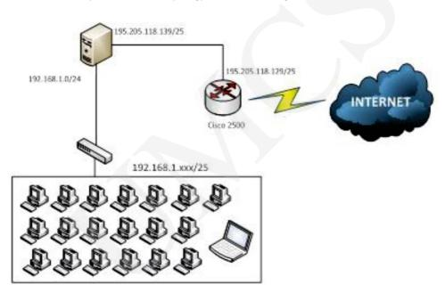
Fig. 1. Analyzed network architecture model.
