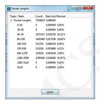
Fig. 2. Examplary statistics of packets lengths in the collected data.
