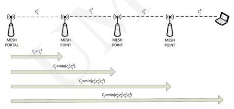
Fig. 2. Throughput in mesh networks.
