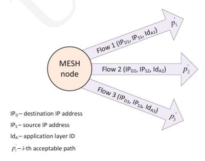
Fig. 9. Hashing Function – Load Balancing.
