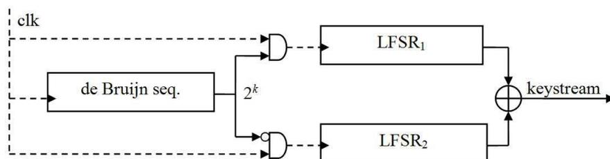
RYSUNEK 1. The Alternating Step Generator
