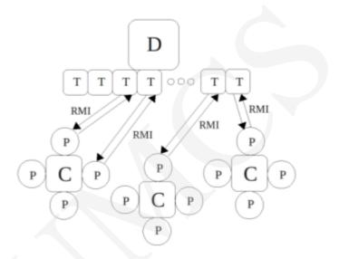
Figure 2 Implementation of the distributed processing model
