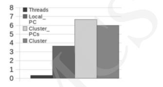
Figure 5 Comparison results of time needed to transferring data between the tasks dispatcher and 3 workers averaged from all attempts [ms]
