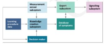
Fig. 2 An attack detection system model
