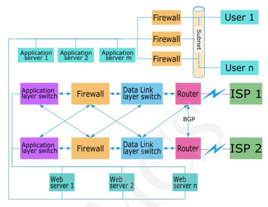
Fig. 2. Architecture of an elaborate firewall
