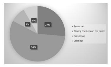
**Figure 8.** The share of individual times of operations performed during the picking process Source: Authors' own study.
