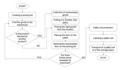
**Figure 7.** The picking process before the change
