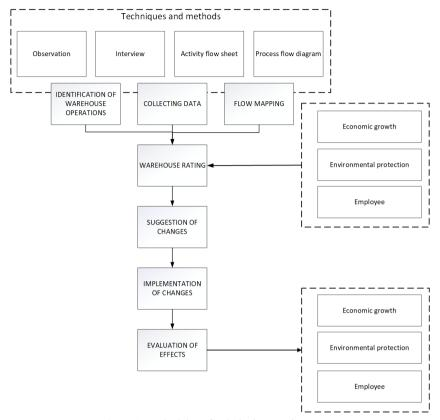
Figure 1. Methodology for designing warehouse space
